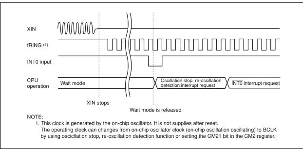
Figures 22.1 and 22.2 show the operation timing at oscillation stop, re-oscillation stop detection.
